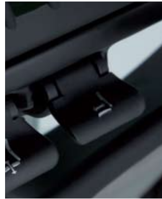
sliding seat adjustment
